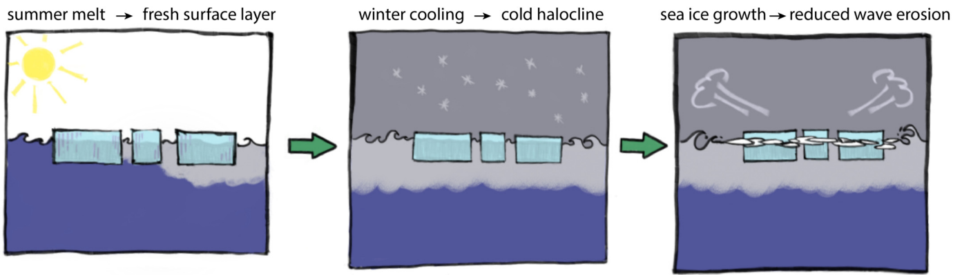
Fig. 4. Proposed mechanism for prolonged iceberg lifetimes. Left: summer melt of icebergs creates a shallow fresh surface layer. Middle: As temperatures drop during fall, the fresh surface layer remains lighter than the saltier waters below. Right: This allows for sea ice to grow as the temperature of the surface layer drops below freezing, which in turn protects the icebergs from wave-induced sidewall erosion and prolongs their lifetimes.
